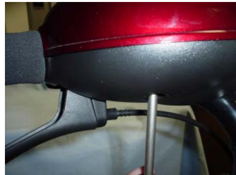
1. Remove the top of the tiller.
