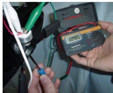
3 & 4. Using a digital multimeter, re-calibrate the throttle potentiometer.
